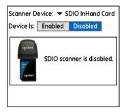
4. The screen will display a picture of the Cordless Hand Scanner. In the Device is field, tap Enabled.
